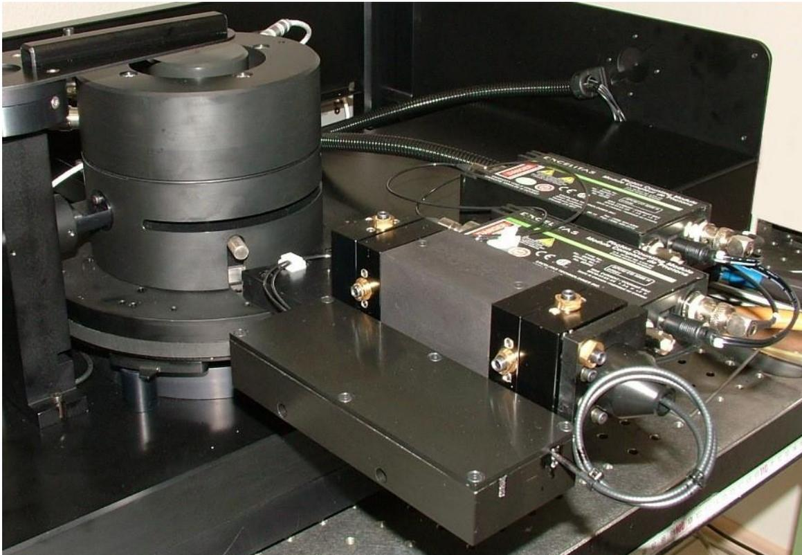
Detection unit with PseudoCross Correlation Setup consisting of two ALV-High Q.E. APD units
